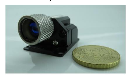
• The uniqueness of this compact size laser is that the beam points at wavelength of 532nm(green).
